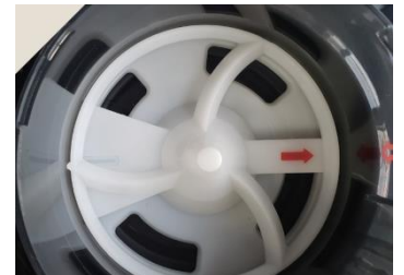
4. Installation the powder mixing turntable.
